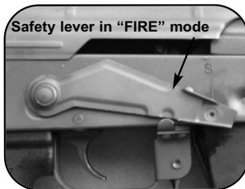
**Safety lever in lower or "FIRE" position. Pulling the trigger when the safety lever is in the lower position will result in the rifle firing if there is a round in the chamber! Exercise extreme caution when handling the rifle in this condition.**
