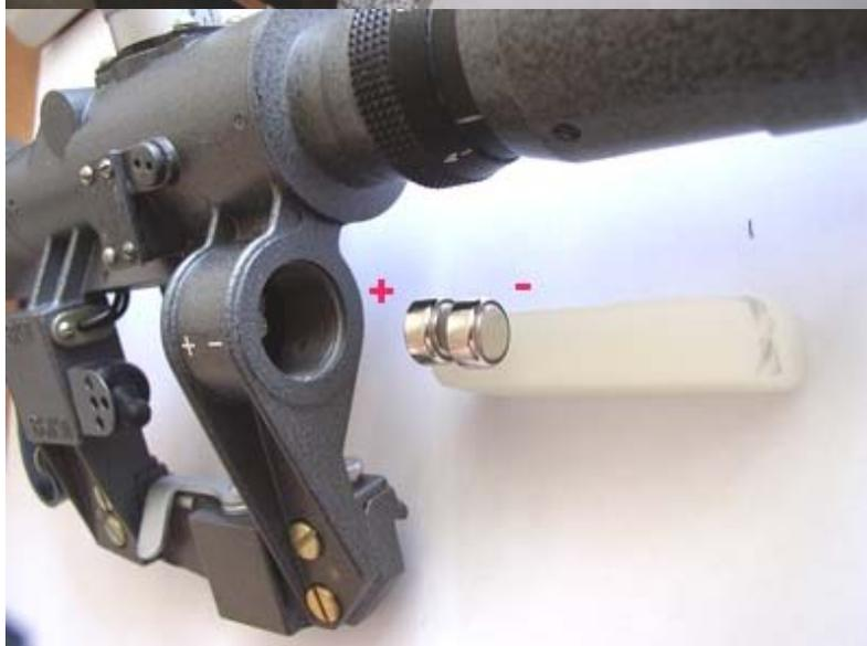
3. Connect the battery and the housing of the sight by metal tool (for example, by tweezers). If illumination began to work, the reason is bad contact between the spring and the cover of batteries housing. If illumination does not work, check up the LED.
