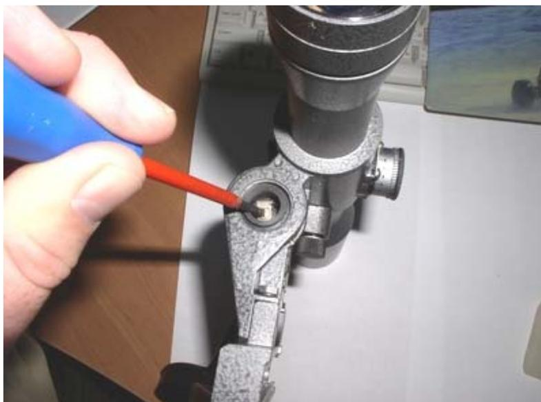
2. Insert batteries as shown in figure. Use only AG13 (or LR44, #357) batteries. (**Attention!** For the PK-A scope "+" should be outside.)
