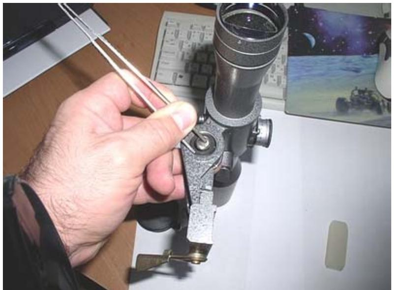
4. For LED check is enough to have good batteries and a paper clip.
